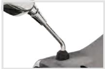
New mirrors design with better fixing of the mirror stems to the handlebar.
