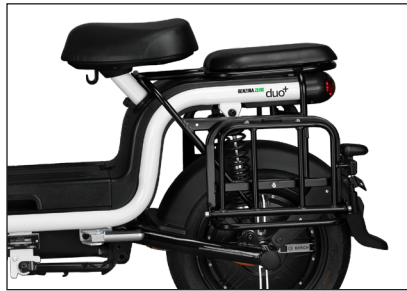
Rack Rear Foldable — Part #: FBS01001038 Pillion Seat Cushion — Part #: FBS01002008 Footpeg Rear L/H — Part #: 84B20-CK02-00000 Footpeg Rear R/H — Part #: 84B10-CK02-00000
